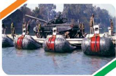
Float for KM Bridge
